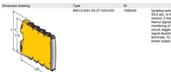
Isolating switching amplifier, 2-channel; SIL2 acc. to IEC 61508; Ex-proof version; 2 transistor outputs; input Namur signal; ON/OFF switchable monitoring of wire-break and short-circuit; toggle between NO/NC mode; signal doubling; removable screw terminals; 12.5 mm wide; 24 VDC nower supply
