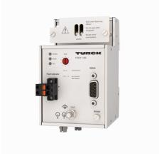
The FOC11... fiber optic media converter converts RS485 signals, e.g. from PROFIBUS-DP or Modbus RTU, on copper cables into optical signals and vice versa. Bus signals from the safe area up to zone 1 can thus be transmitted intrinsically safe, potential-free and interference-free over long distances.
