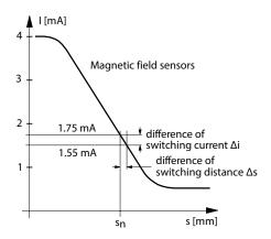
Abb. 1: NAMUR characteristic curve of the magnetic field sensors in compliance with EN 60947-5-6
