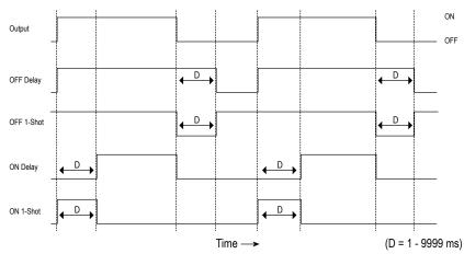
Figure 18. Delays/Timers
